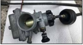
While I was waiting, I turned my attention to getting it running. First up, drain and replace the oil from the engine and the oil tank, and inspect the fuel tank for rust and the carburettor for sludge. Both were so bad, I ended up taking them to
